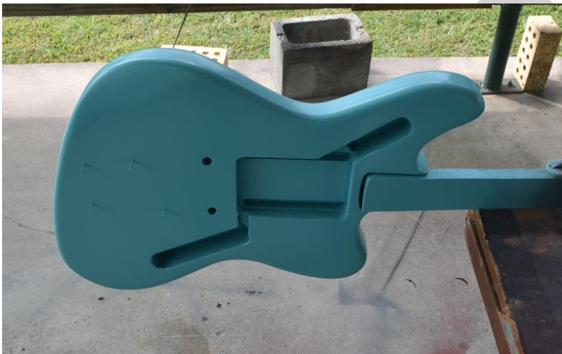
A handy way of holding a body for painting or staining is a piece of timber attached in place of the neck. (notice the tooth picks used to block screw holes)
